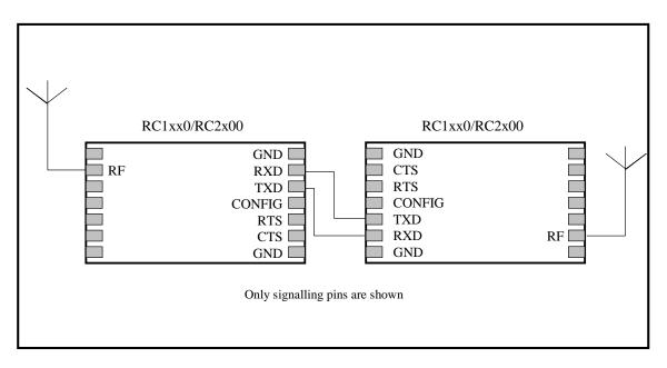
The second module will then re-transmit the incoming packet on what can be seen as a secondary network, which can be on another frequency or on the same frequency but with different addressing. This simple repeater will in practice double the range when inserted in a link for repeating purposes.
