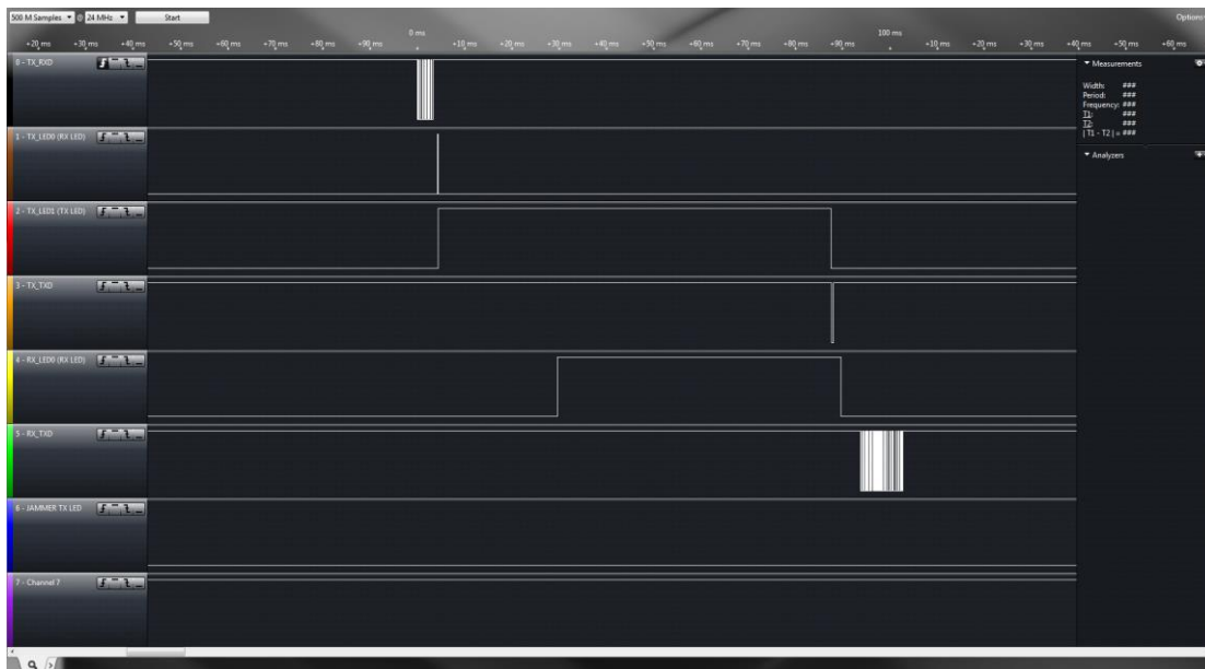
Figure 1. LBT with no jammer. Message is sent immediately.
