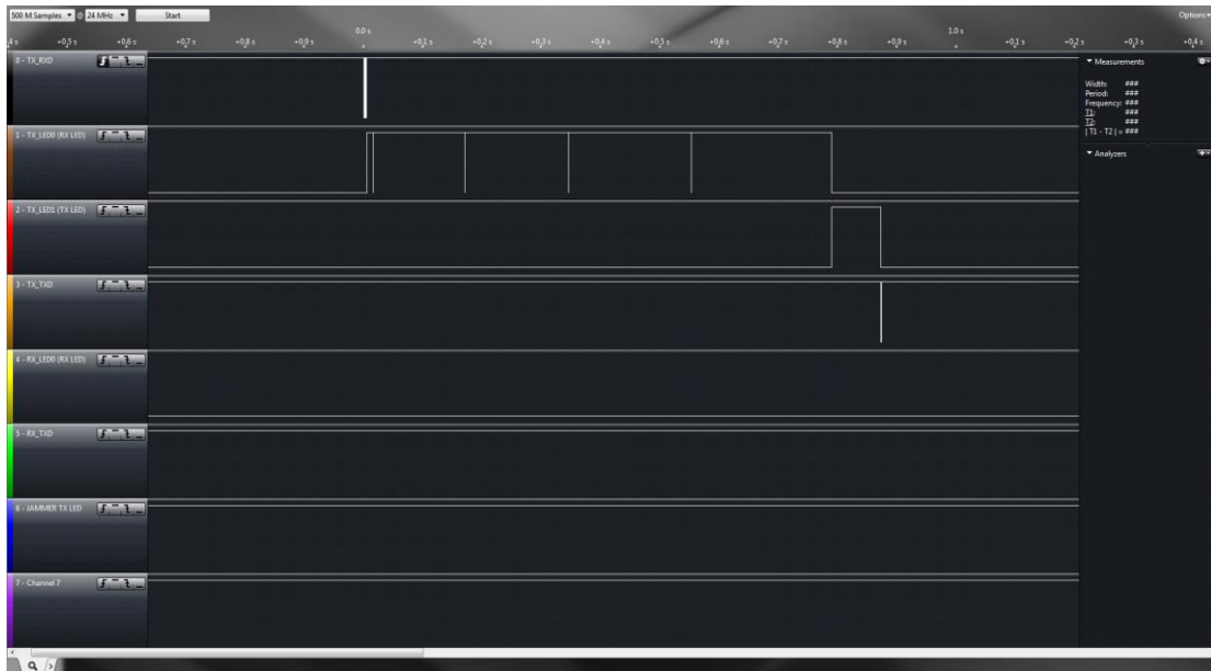
Figure 3. LBT with jammer. Message is sent by override.
