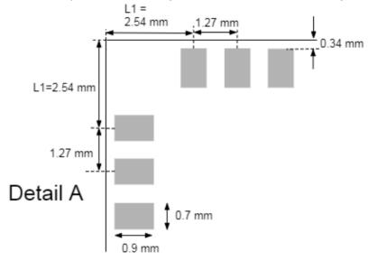
If there is a need to use wider CPW then this interface should be done with a taper or curved taper onto the module. A sudden change in width means a sudden change in transmission line impedance. This will give reflections, lower output power and less than optimal performance. [2]
