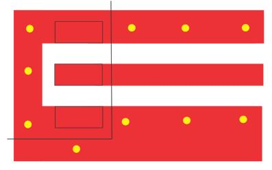
Vias inside the pad may lead to reliability issues when soldering the module in place. The recommended approach is to have the vias outside the solder pad.
