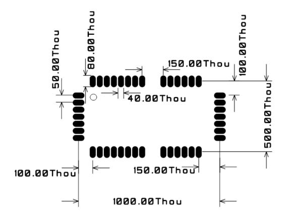
A PCB with two or more layers and with a solid ground plane in one of the inner- or bottom layer(s) is recommended. All GND-pins of the module shall be connected to this ground plane with vias with shortest possible routing, one via per GND-pin.
