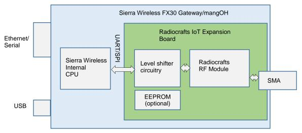
Figure 1: Functional block diagram for FX30 gateway and IoT expansion board
