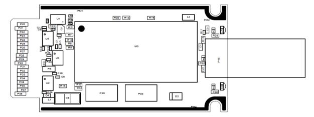
Figure 6: RCxxxx-IEB PCB component placement, top side
