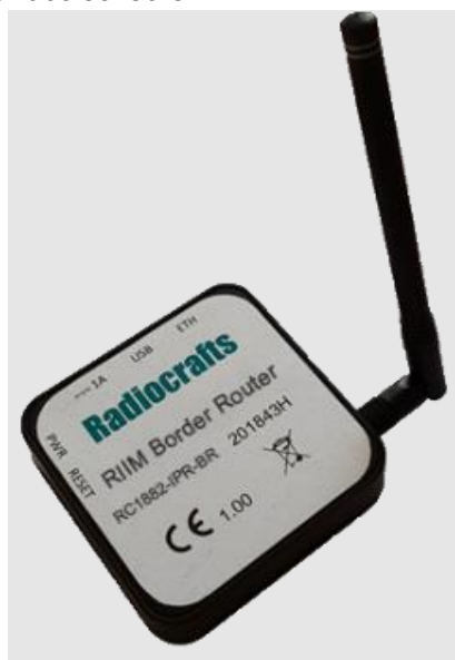
Figure 12. Radiocrafts off-the-shelf border router
